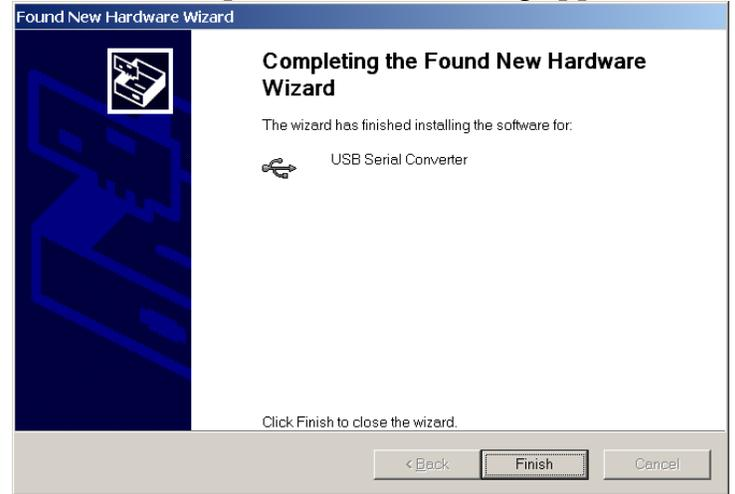
Click *Finish*... but we are not done! The first phase installs the USB driver, the second, a virtual serial port driver. The following message appears:
